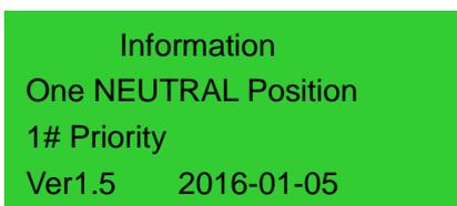
Display contents include current breaking positions setting, transfer priority choice and controller version and date.
