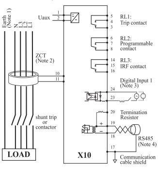
Note 1: The EARTH wire must not pass through the ZCT.
