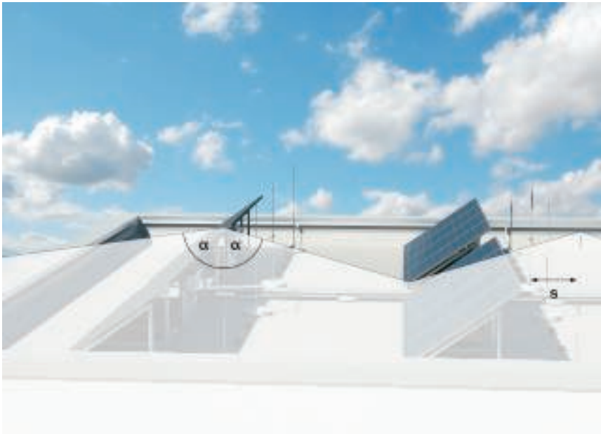
\alpha^\circ = lightning protection angle, s = separating distance
