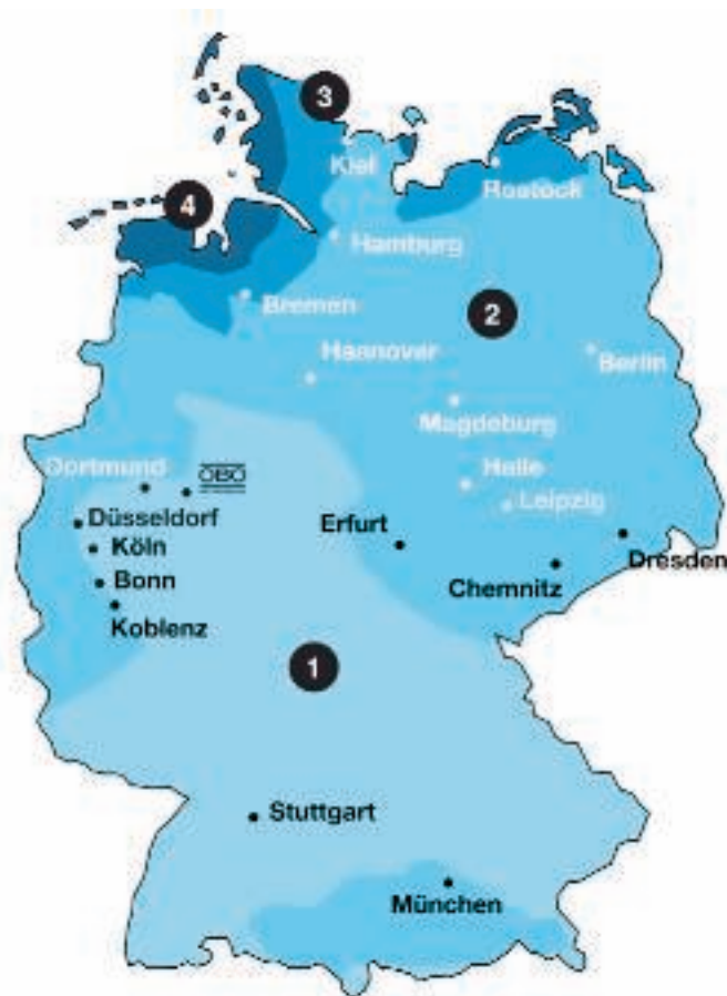
Wind load zones in Germany according to DIN 1055-4
